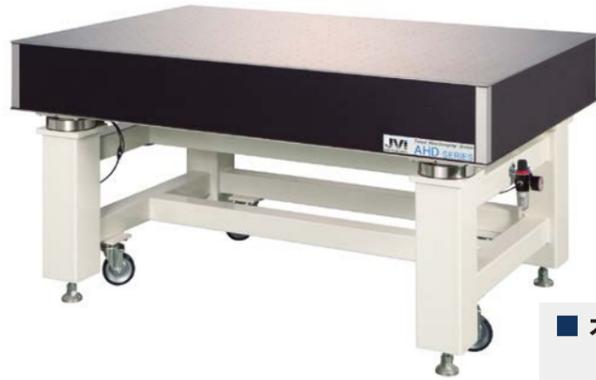
AHD series are used the High Grade Damping Steel Honeycomb table with a built-in Tuned Mass Damping-system (TMD). When used with the Omni Directional Three-dimensional Air Spring System, AHD series can provide high level of vibration isolating performance. We realize to eliminate the resonance peak because JVI design the original TMD by each vibration mode. Also, the damping of surface table reduces the resonance of the work-surface. The drop-preventive bottom structure is standard equipment.
