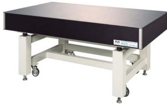
The Standard Damping Steel Honeycomb table with a built-in Tuned Mass Damping-system (TMD) combines the Rubber Vibration Isolating System. We realize to eliminate the resonance peak because JVI design the original TMD by each vibration mode. RSD series are resulted from the pursuit of both RHD's damping effect and high cost performance
