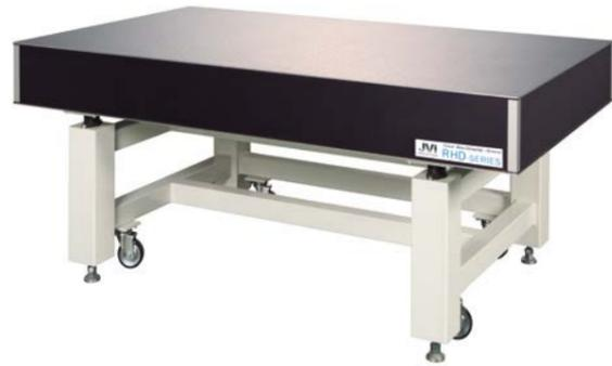
The High Grade Damping Steel Honeycomb table with a built-in Tuned Mass Damping-system (TMD) combines the Rubber Vibration Isolating System. We realize to eliminate the resonance peak because JVI design the original TMD by each vibration mode. Also, the damping of surface table reduces the resonance of the work-surface. The drop-preventive bottom structure is standard equipment.
